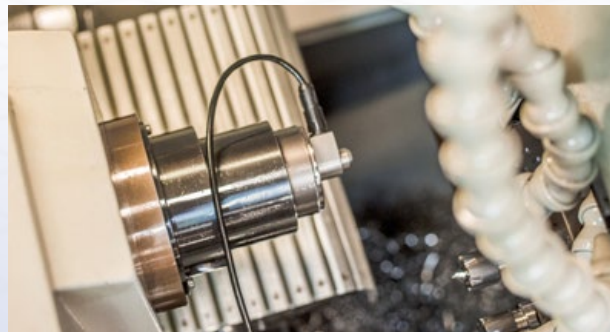
Camera in sub spindle,
